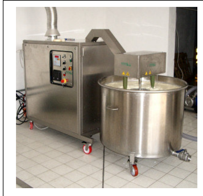
POLYFOOD WITH SDR (patent EP 774895 and US 5916352) maximum thermal exchange = 6 °/minute
