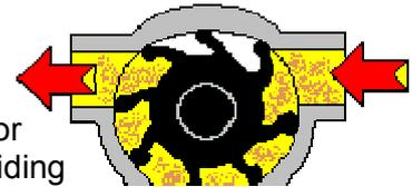
The pump can operate in both rotation directions, which permits return of excess liquid without any manual intervention, and also allows easy emptying of pipes on completion of liquid transfer.
